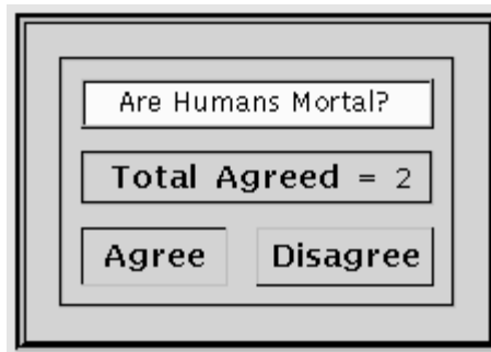
FIGURE 3.1 A simple groupware application: A polling program. This example illustrates how shared and private views can co-exist in Multi-User Clock applications. In this application, while the views pertaining to the proposition and the poll result are shared by all the users, the view of the radio buttons is private for each user. The private views in this application are intended to maintain the anonymity of the users.
