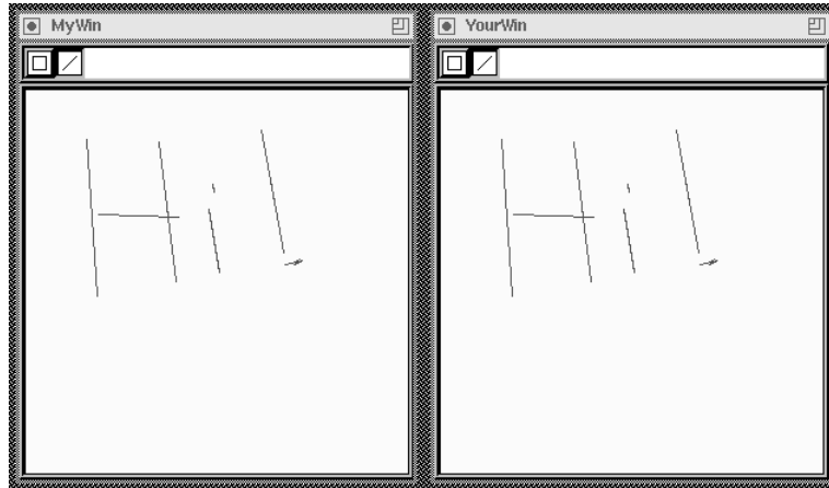
FIGURE 2.1 An example of a Groupware application: A shared drawing program. The figure illustrates two windows, each of which belongs to one user of the program. The objects drawn by each user are depicted on all users' displays.
