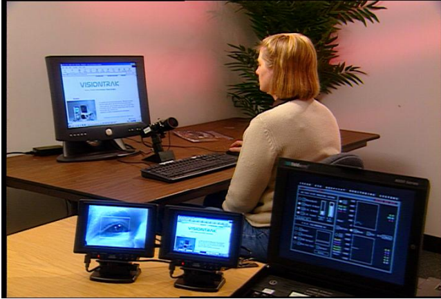
Figure 3: The Polhemus VisionTrak ETL-400 uses a camera and an IR light source situated around the camera lens to track the user's eyes [17].
