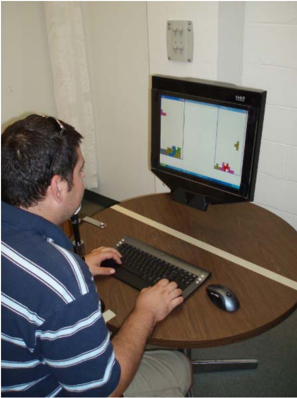
Figure 4: Experimental set-up: a Tobii eye tracker is used to determine where the players are looking during experiments.
