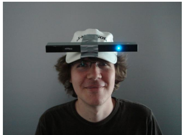
Figure 3. Head-tracking using sensor bar.
