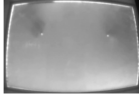
Figure 2: Example of raw camera input. Two touches show as bright white spots, with nearby shadows.
