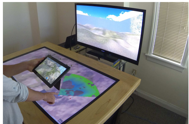
Figure 1. TerraGuide. The interactive tabletop provides the user with a 2D top-down view of a 3D terrain. Viewsheds show visibility from a source point. A secondary display shows a panoramic view. A hand-held tablet displays terrain in 3D.
