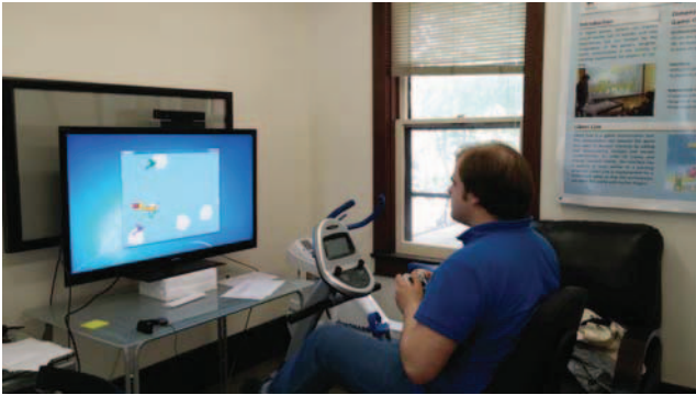
Fig. 2 Study setup. The player sits at the exercise bike, and holds the game controller. The game appears on the television screen.
