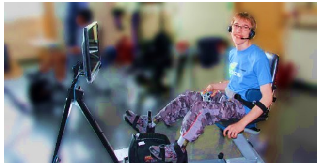
Figure 1: Youth with CP seated on custom-built recumbent bicycle with pedaling attachments and lateral supports.
