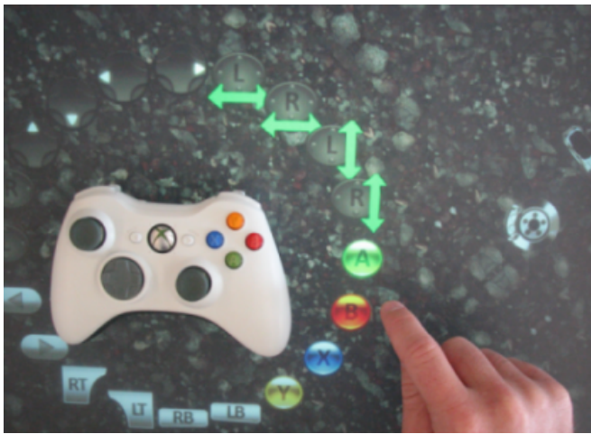
Figure 4: When an Xbox 360 controller is placed on the table, a ring of “pins” surrounds the controller showing its various outputs. These pins can be connected to inputs on interactive objects.
